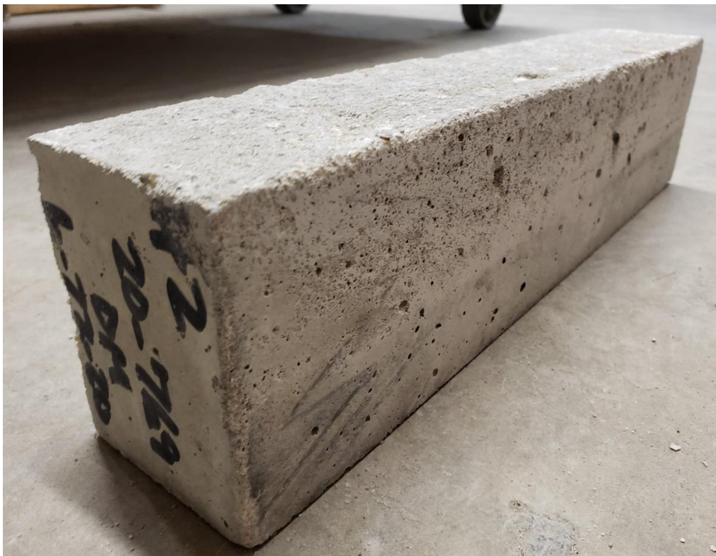
Photo #2 – Freeze/Thaw Beam After 300 Cycles
